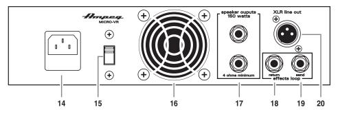
14. IEC POWER INPUT CONNECTOR: This is where you connect the supplied AC power cord.
